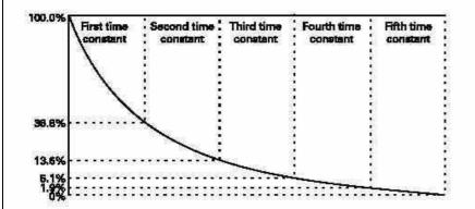
CALCULATING THE TIME CONSTANT OF AN INDUCTIVE CIRCUIT:
