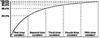
CALCULATING THE TIME CONSTANT OF A CAPACITIVE CIRCUIT:
