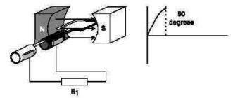
GENERATION OPERATION FROM 90 TO 180 DEGREES: The armature continues to rotate from 90 to 180 degrees, cutting less lines of flux. The induced voltage decreases from a maximum positive value to zero.
