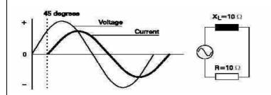
When working with a circuit containing elements of inductance, capacitance, and resistance, impedance must be calculated. Because electrical concepts deal with trigonometric functions, this is not a simple matter of subtraction and addition.
